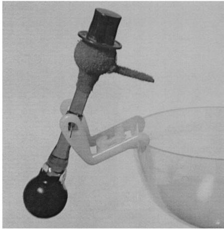
Fig. 1. Schematic and photo of our sunbird (drinking bird with a black-painted body) illuminated by a conical light bulb. A screen prevents the head from being illuminated. The glass is empty. Compare with Fig. 1 of paper I.
