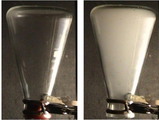
**Figure 2.** Fog in a bottle. The pressure is increased inside the bottle. When the cork flies out of the bottle, the abrupt decrease in the pressure originates a cloud. The experiment works better if few drops of water are placed inside the flask (as suggested by Coop [10]).
