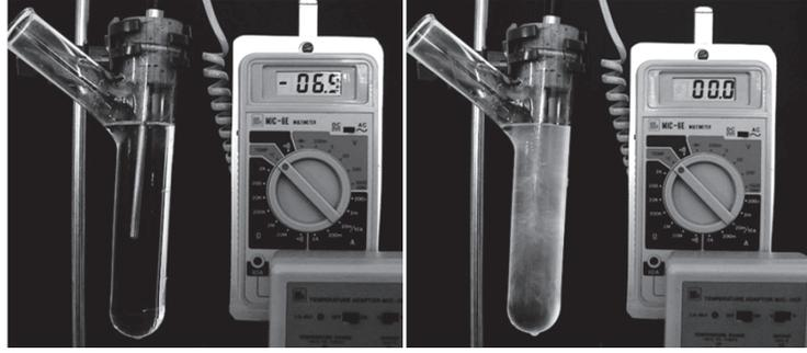
**Figure 2.** Supercooled water. A test tube with bidistilled water was introduced into a receptacle containing a mixture of saturated salted water and ice below the freezing point (on the left). When crystallization occurs, the temperature increases to 0 °C (on the right).
